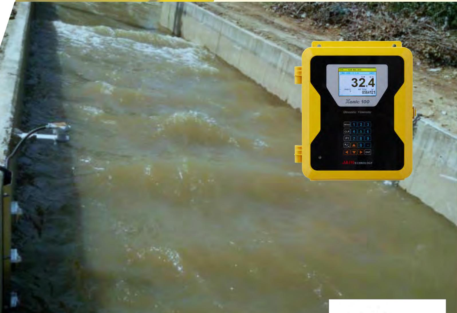
Xonic100LM Ultrasonic Open Channel Flowmeter use ultrasonic transit-time method for flow velocity and use level meter to receive level data. Xonic 100LM not only measure velocity, but measure sound speed and can compensate temperature change by it's own diagnostic functions. Xonic 100LM is newly developed and has very sophisticated diagnostic functions for better performance.
