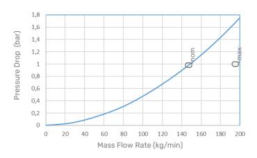
0 – 200 kg/min water, sensor with P1 pressure rating. Higher viscosities create higher pressure drop
