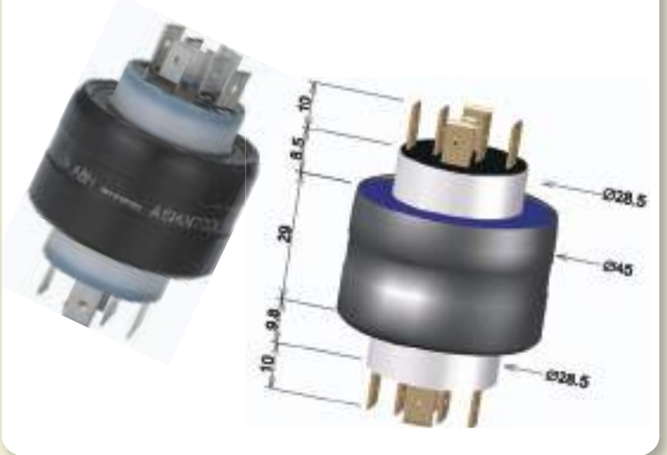
A8H NM (non-mercury) 6poles/30A & 2poles/4A AC250V
