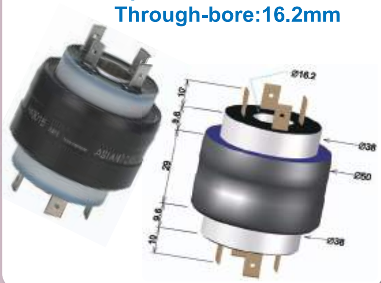
H63016 6poles/30A/AC250V Through-bore:16.2mm
