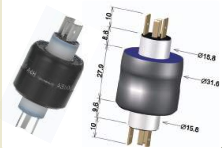
A4H NM (non-mercury) 2poles/30A & 2poles/4A AC250V
