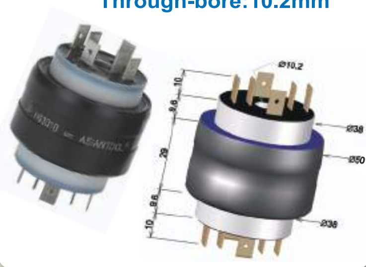
H103010 10poles/30A/AC250V Through-bore:10.2mm
