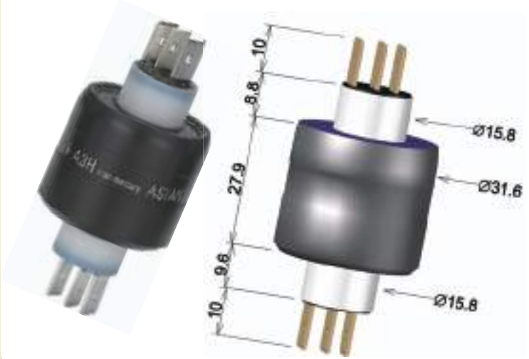
A3H NM (non-mercury) 3poles/30A/AC250V
