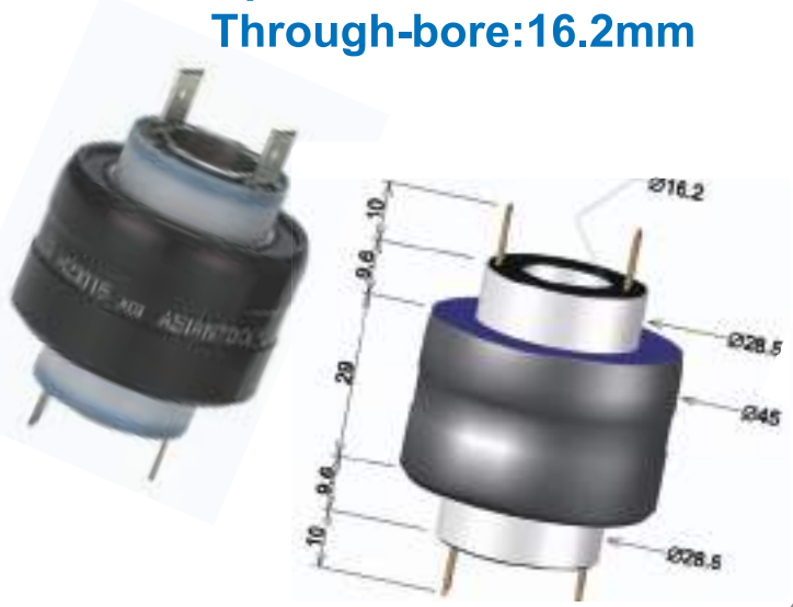
H63016 6poles/30A/AC250V Through-bore:16.2mm
