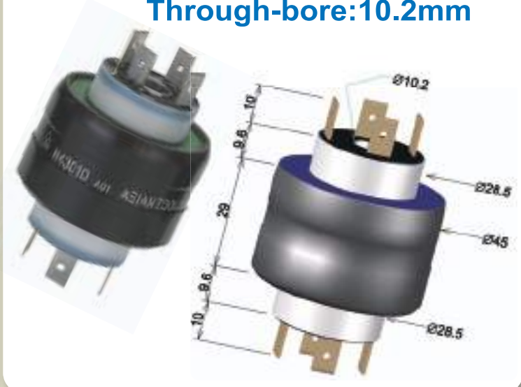
H83010 8poles/30A/AC250V Through-bore:10.2mm
