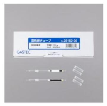
The activated carbon tube is used in work environments where organic-solvent vapour is collected. Generally the activated carbon tube is suited for detection of almost all organic solvents of low polarity .
