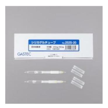
The silica gel tube is used in work environments where organic-solvent vapour is collected. Generally the silica gel tube is suited for substances of high polarity (e.g. acetone, methanol, etc.).
