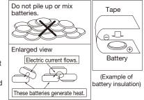
so make sure to cover the (+) and (–) terminals with friction tape or some other insulator before disposal.
